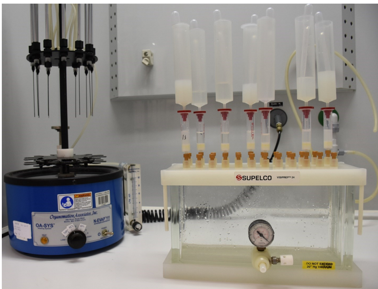
Figure 6. Tetracycline extraction - SPE cartridges with C18 packing positioned on the Vacuum manifold. Slika 6. Ekstrakcija tetraciklina – SPE kolonice s C18 nosilcem so postavljene na Vacuum manifold.
