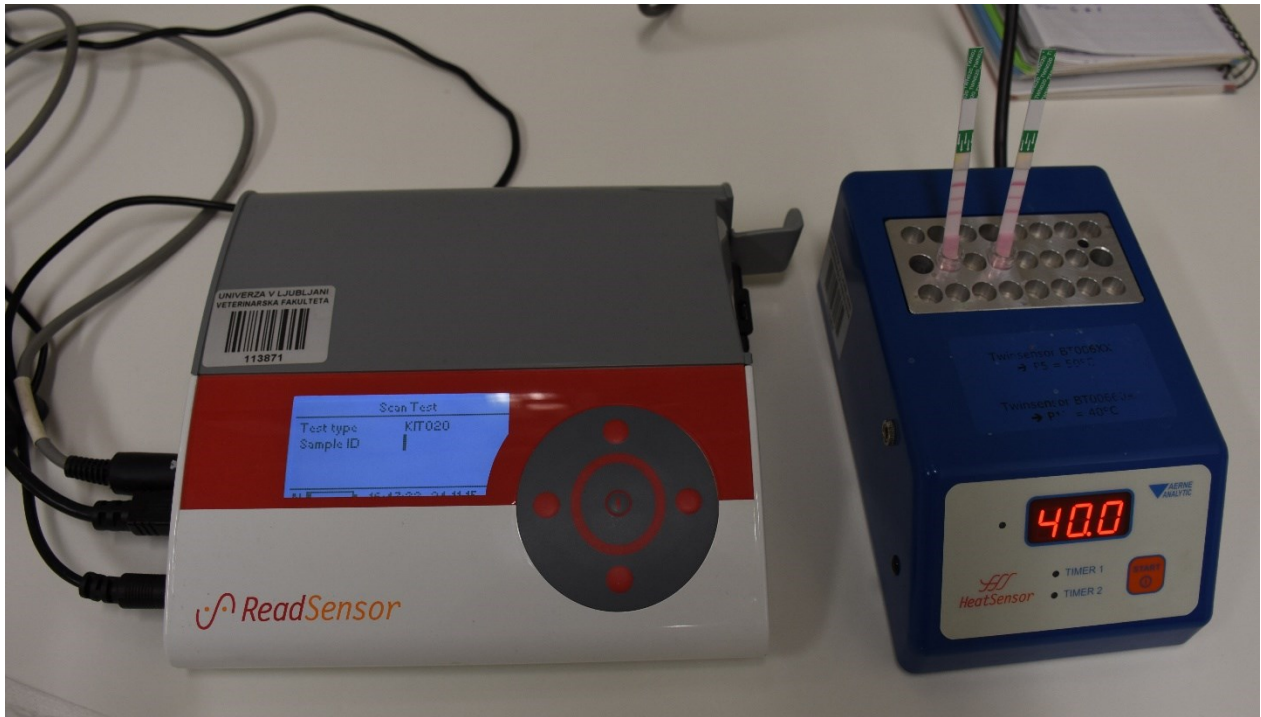
Figure 4. Heatsensor (right) with two dipsticks and Readsensor (left). From the picture it can be noticed that both dipsticks are negative on penicillins and cephalosporins.
